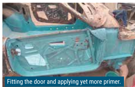
The offside door is treated to a new skin.
