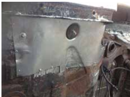
With the rot cut away, new metalwork was tacked in place before Paul got to work with his welder.
