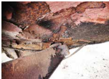
The underside was very rusty, as shown with this passenger-side rear radius mount.
